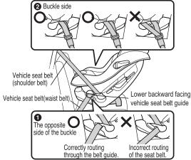
Press onto the main body of the child car seat and tighten vehicle seat belt(shoulder belt) so as to remove any looseness on the vehicle seat belt(waist belt).
