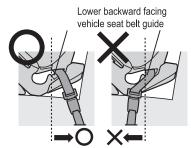
If the extension point of the vehicle seat belt is located in front of the backward facing seat belt guide(lower) installation may
